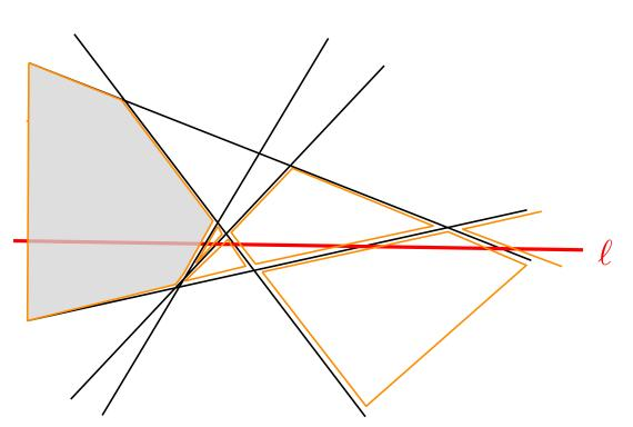
Cost of threading  $\ell$  into  $\mathcal{A}(L')$ : 1. O(n) for locating cell of  $\mathcal{A}(L')$ , where  $\ell$  starts "from the left" 2. O(sum of the sizesof the cells intersected by  $\ell)$  $= O(z(\ell, L')) \leq 6n$
