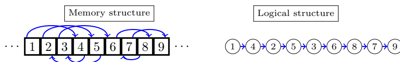
Figure 1.2: State after many insertion and deletion operations. There may also be “dead” cells which are currently not part of the list. These are not shown; we assume that these are taken care of every now and then to avoid wasting too much memory.
