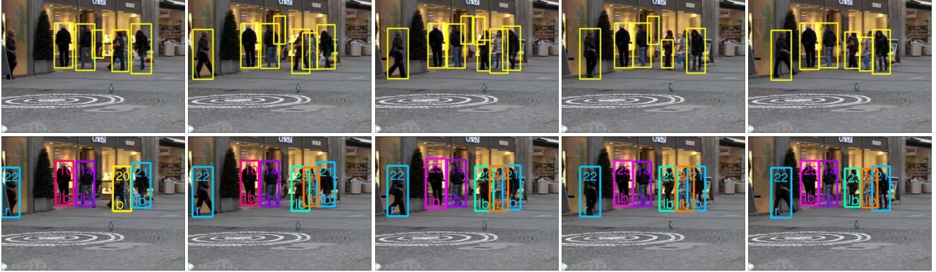
Figure 5. People detection based on single frames (top) and tracklets found by our 2D tracking algorithm; Different tracklets are identified by color and the estimated viewpoints are indicated with two letters (bottom). Note that several false positives in the top row are filtered out and additional – often partially occluded – detections are filled in (e.g., on the left side of the leftmost image).
